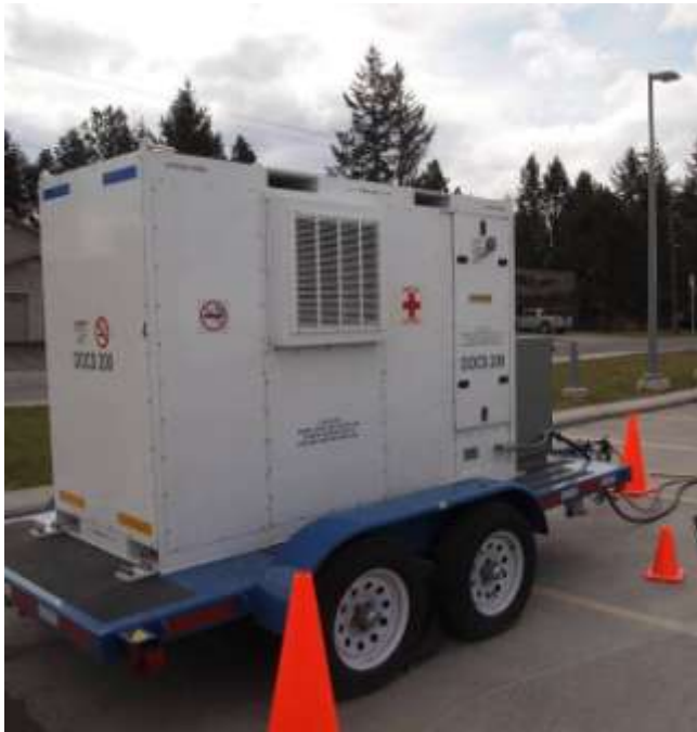
Portable oxygen generation system – 95% O 2
