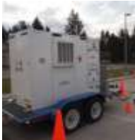
Portable oxygen generation system – 95% O 2
